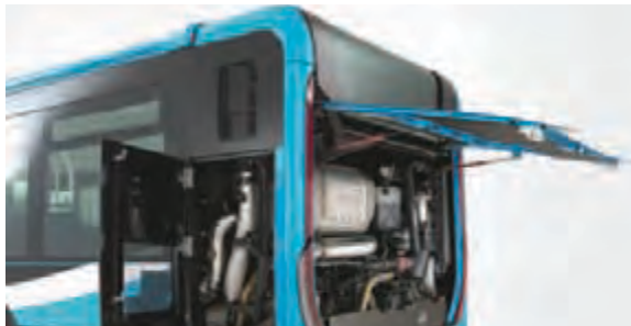
The engine compartment can be easily accessed via several quick-open panels.
