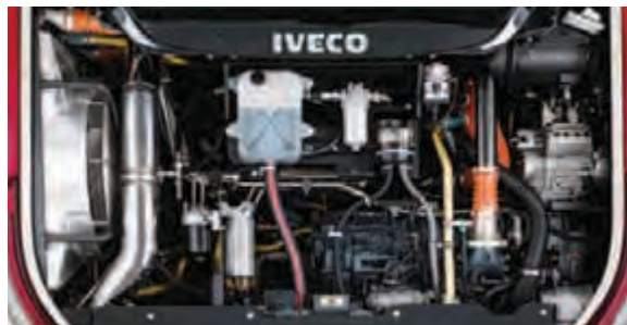
Filters and tanks are grouped together to simplify daily checks.
